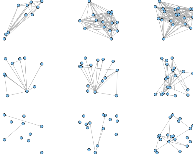
Figure 2.4: Examples of the output of network growth models for graphs of 10, 15, and 20 nodes: forest-fire (top row), preferential attachment (middle), random attachment (bottom).
